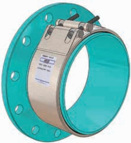
Teekay Flange Adaptors make the installation of pumps and valves quicker and easier. Simply bolt the flange adaptor on to the existing flange and fasten the coupling over the joint between the flange adaptor and plain end pipe. This creates a useful maintenance point in the future: undo the bolts on the coupling rather than the nuts on the flange adaptor and lift out the piece of equipment!
