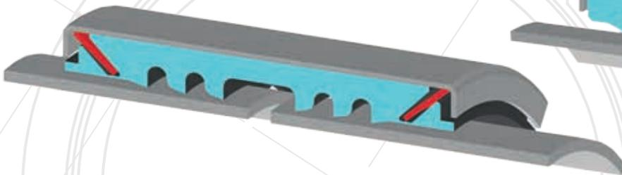
As the lockpart is tightened the sealing lips are pressed against the pipe surface to form a seal. At the same time the anchor rings penetrate the rubber, bite into the two pipes and prevent them from pulling apart, whether by external loading or internal pressure. The end seal is also pressed against the pipe surface, which protects both the anchor ring and the section of the pipe where the anchor rings have bitten, from any possible external corrosion.
