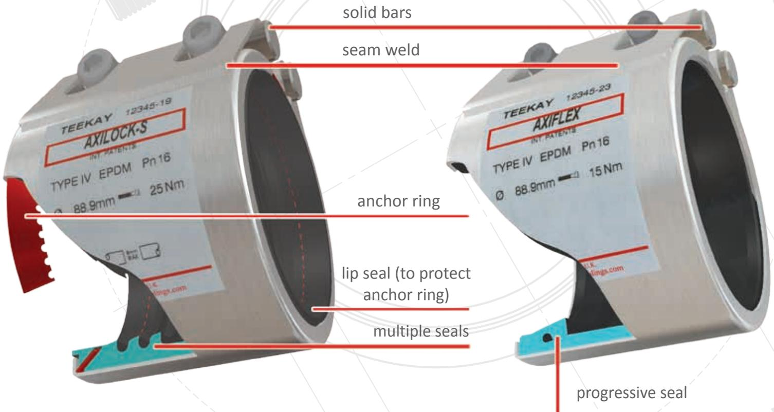
Each coupling (whether **Axilock** or **Axiflex**) consists of a casing, a gasket and a lockpart. The purpose of the casing is to house the gasket and to press it onto the pipe surface when the lockpart is closed. The lockpart is designed to pull the two ends of the casing together circumferentially around the pipe. In order to achieve this, the coupling is labelled clearly with a torque figure which ensures that the gasket is compressed sufficiently against the pipe surface.
