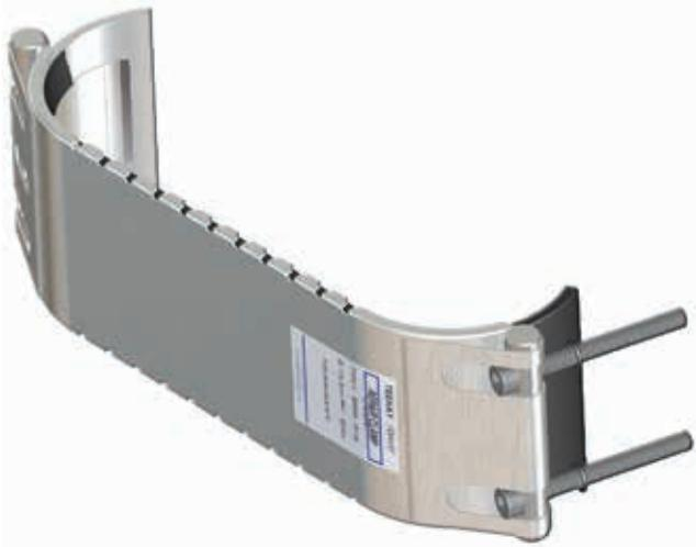
The Teekay Repair Clamp is the budget repair coupling of choice. Featuring “cut flanges” on the underside of the fitting, this type of coupling can be easily pulled around a leaking pipe to seal a fracture. Once wrapped around the pipe, the fitter then goes about installing the coupling in the same manner as any other Teekay coupling.
