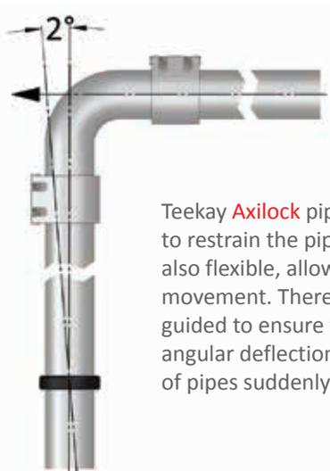
Teekay **Axilock** pipe couplings are designed to restrain the pipes axially. However, they are also flexible, allowing some axial and angular movement. Therefore the pipes should be guided to ensure that they remain within 2° angular deflection, especially where a long run of pipes suddenly changes direction.
