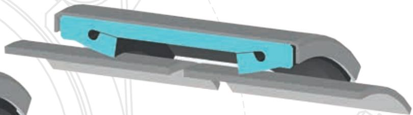
The sealing lips press against the pipe surface and form lip seals. The lip seals are designed to resist the internal pressure in the pipes. As the pressure increases, the lip seals swell to seal more tightly against the pipe surface.
