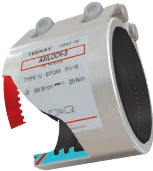
The Teekay Axilock range is designed to replace the need for flanging, welding, pipe grooving and pipe threading by providing a quick and easy solution to joining plain-end pipe. Incorporating grip rings at each end of the fitting, the Teekay Axilock offers high levels of security by locking the pipes together under pressure. Each coupling is 100% rubber-lined, ensuring that high levels of corrosion resistance are maintained throughout the life of the coupling.
