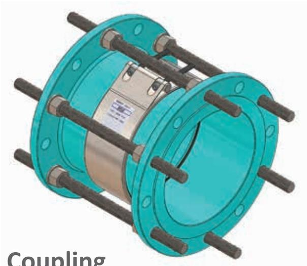
Teekay Dismantling Joints facilitate the easy access and removal of equipment when it comes to long-term maintenance of piping systems. Rather than moving large sections of fixed pipework, use the Dismantling Joint to create space and easy access to pumps, valves and flowmeters.
